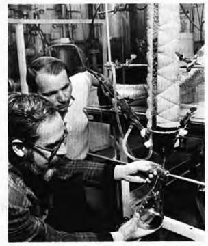
USING LAB APPARATUS, Charlie Arnold (5811) and Dick Curlee (5843) simulate oil shale in-situ processing. The asbestos-covered glass tube contains oil shale rubble which has been ignited at top. As the rubble burns down, oil collects at bottom
